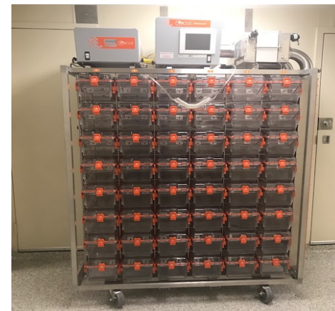
Four bio-containment racks (48 cages each)
